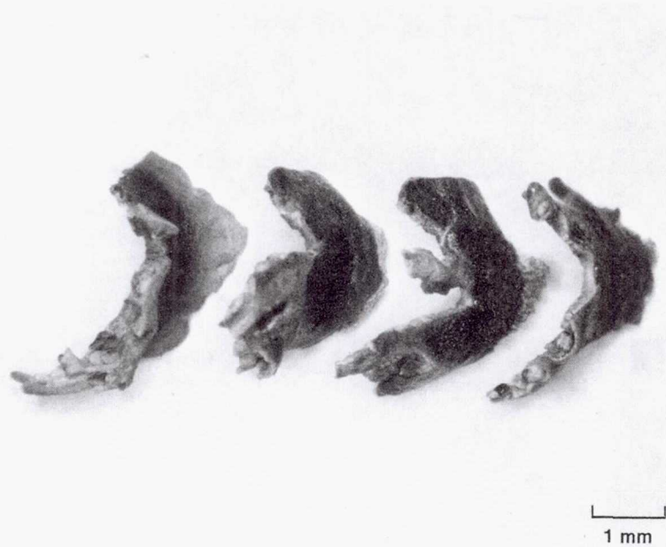
Figure 5.—Macrograph of four leading edge vane deposits showing viscous flow patterns around sides.
