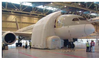
A Boeing 787 fuselage repair shelter set in in Doha, Qatar.
