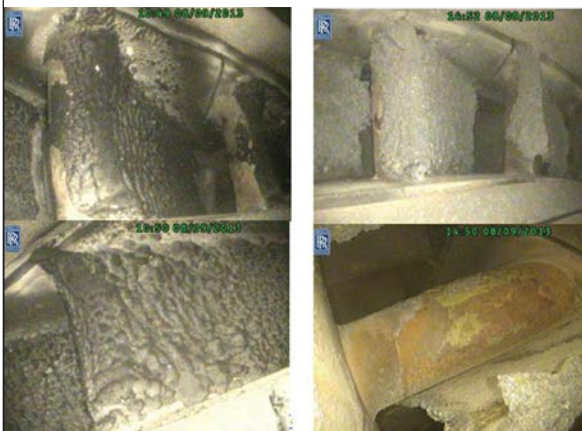
Turbine vane blades of the left-hand engine (left) of the MV-22B that was written off after an August 2013 hard landing and fire at Creech AFB, Nevada, show the glasslike accretion of melted particles that reduced airflow and caused the engine to surge. The right-hand engine (right) was not as badly affected.
