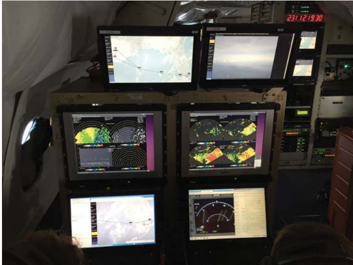
To evaluate standard radars for HIWC warning, Honeywell RDR-4000 weather radar data was collected from simultaneous scans above, level and below the flight path and compared with data from the ice-measuring instruments.
