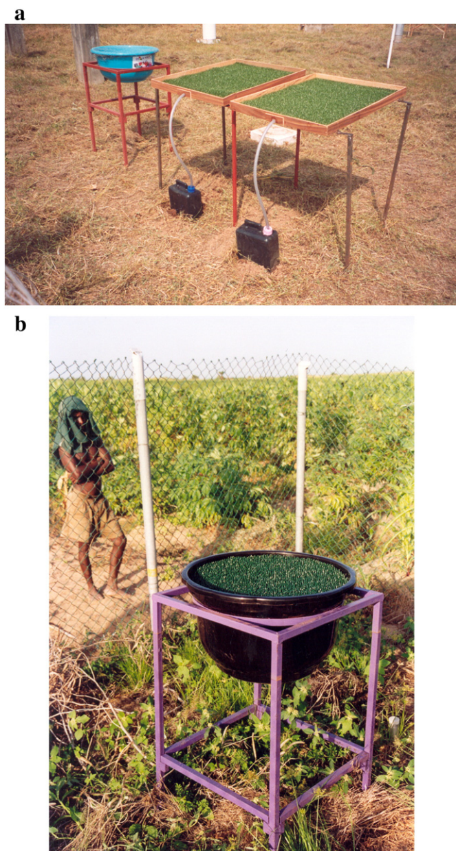
Fig. 2. Picture of the bowl and mat sampler (a) and bowl-mat (b) used at the sampling sites.
